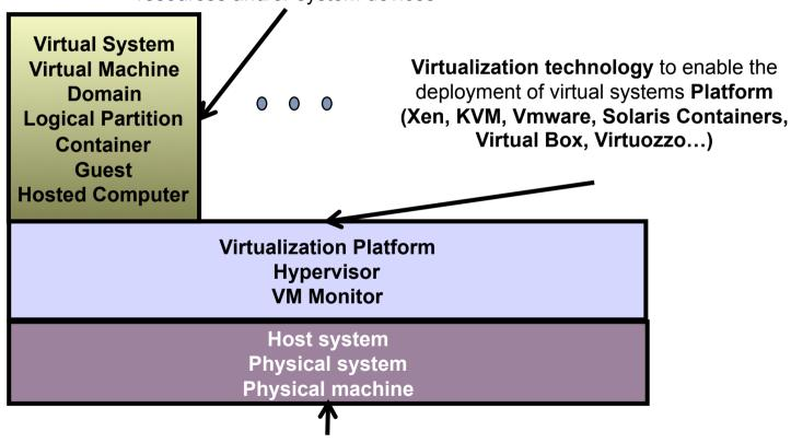
Virtualization environment containing computing resources and devices that are capable of being virtualized
