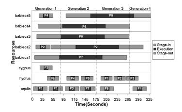
Fig. 2. Execution profile of four generations of the GOGA, each subpopulation has been labeled with  $P_{deme}$
