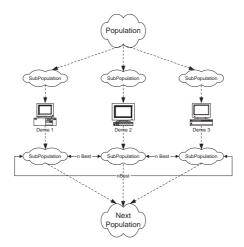
${\bf Fig. 1.}$  Schema of fully-connected multi-deme genetic algorithm, with three computing nodes
