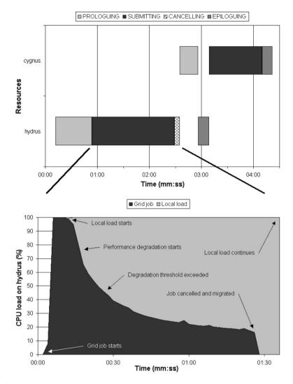
Fig. 1. Execution profile (top) and CPU load on hydrus (bottom) when a migration is performed due to a performance degradation.
