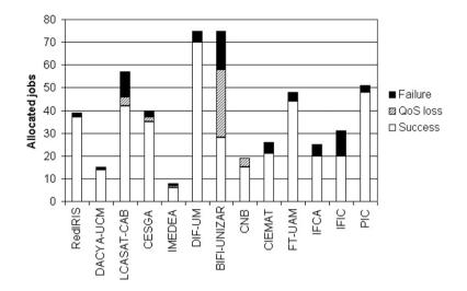
Fig. 3. Distribution of total successful executions, failure conditions and QoS loss conditions across sites.
