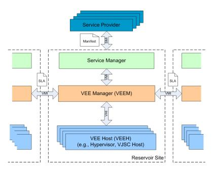
Figure 4: The RESERVOIR Architecture: major components and interfaces
