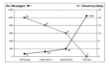
Fig. 3. Bandwidth consumption and discovery delay results
